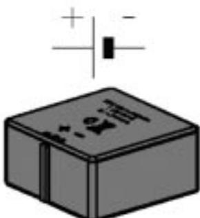
For economic reasons, the use of batteries or accumulators is the only meaningful way to supply robots with current. Solar cells or fuel cells are unfortunately not sufficiently powerful to provide practical results with a reasonable amount of expense.
