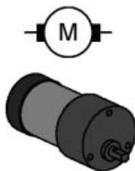
The construction kit contains two different motor types: the mini motor and the power motor. The small, compact mini motor with worm is designed for auxiliary drive or special purposes with small power requirements. It always requires gears for reducing rotational speed.
