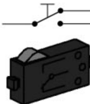
The simple, logical levels "0" and "1" can be depicted using a switch. Precision snap switches are used in the system of fischertechnik construction kits. The special property of snap switches lies in their switching behavior. If you press the red button carefully and slowly, you feel a clear pressure point when the switch contact switches over with a slight clicking sound. If we release the switch
